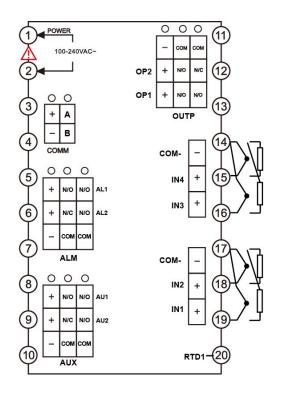
Note: This diagram shows the wiring diagram for vertical panel instruments of types A, C, and E
