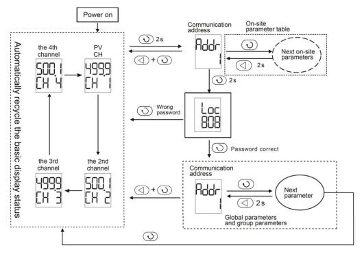
Long press key to enter field parameters; long press key again to view LOC setting 808. Short press key to enter parameter menu; short press key to switch parameters. Press key to exit quickly ( keys must be pressed earlier).
