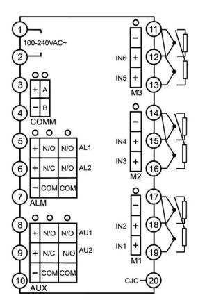
Note: This drawing is the instrument wiring diagram of A/C/E vertical panel
